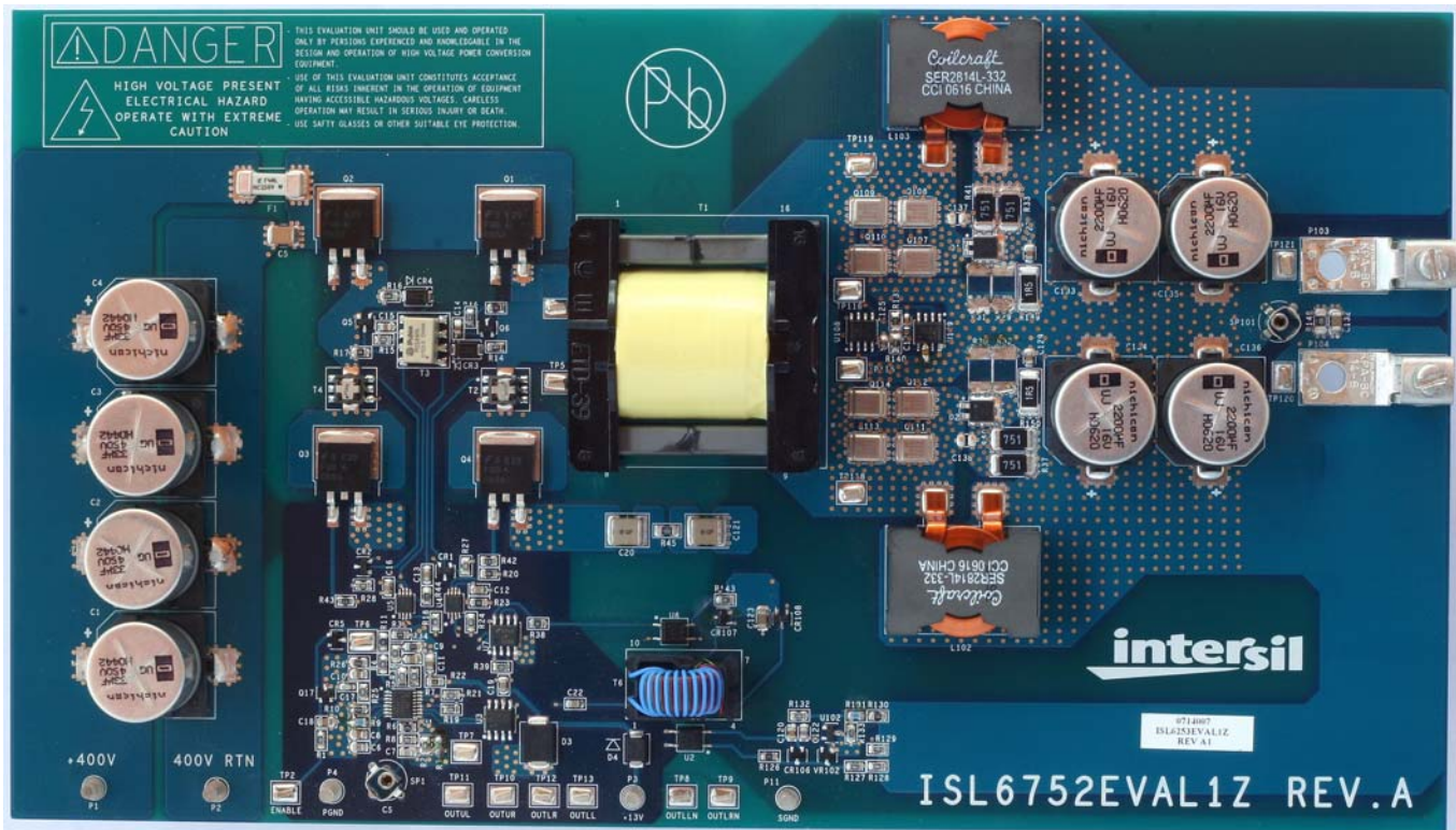
FIGURE 1. ISL6752EVAL1Z EVALUATION BOARD
