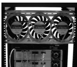
Fig.7 Photograph Showing Three Developed Products Mounted in a 19-inch Rack (EIA standard)
