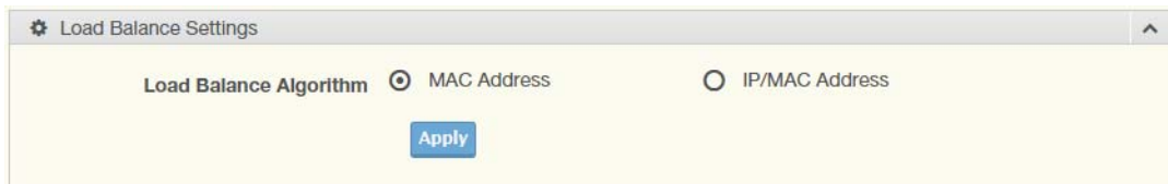
Figure 4.17 L2 Switching > Link Aggregation > Load Balance
