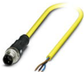
Sensor/actuator cable, 3-position, PVC, yellow, Plug straight M12 SPEEDCON, A-coded, on free cable end, cable length: 5 m
