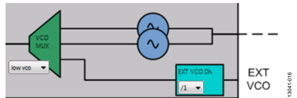
Figure 16. PLL2 Internal External VCO selection
