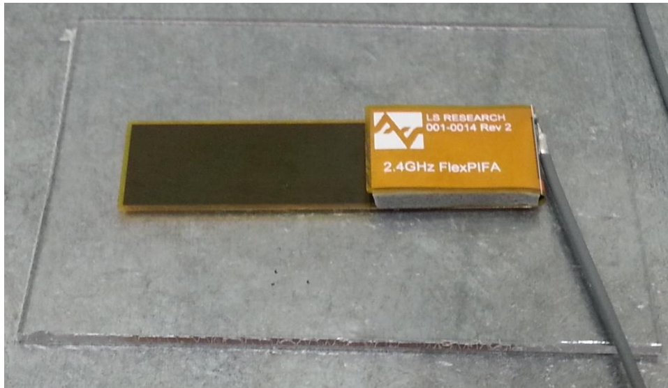
Figure 25 FlexPIFA Mounted on Metal Surface with 1.5mm Thick Polycarbonate Spacer
