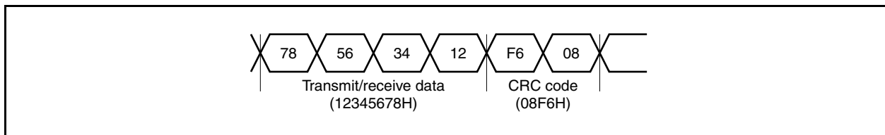
Figure 28-4. CRC Transmission Example
