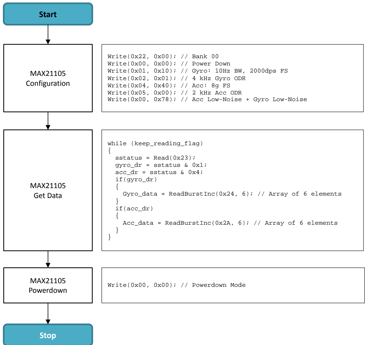
Figure 18: Simple Read-Out Sequence, No FIFO, No Interrupts
