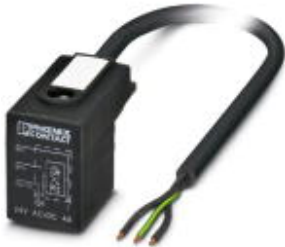
Sensor/Actuator cable, 3-position, PVC, Black RAL 9005, Free cable end, on BI valve plug (11 mm), with 1 LED, connected with Z diode, Cable length: 2 m
