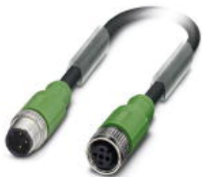
Sensor/actuator cable, 3-position, Variable cable type, shielded, Plug straight M12, A-coded, on Socket straight M12, A-coded, cable length: Free input (0.2 ... 40.0 m)
