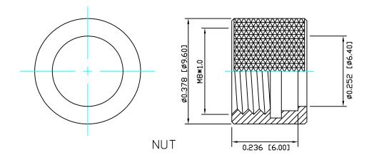
NΠΤF: MATERIAL HOUSING: PBT UL94V-0, BLACK CONTACT: PHOSPHOR BRONZE SHELL BRASS NUT: **BRASS** □-RING: NBR, BLACK FINISH: GOLD PLATED CONTACT: □VER 50 u NICKEL BRIGHT TIN 604" GROUND: SHELL: NICKEL PLATED **ELECTRICAL** RATED CURRENT: 5A 125V RATED VOLTAGE: INSULATION RESISTANCE: 1000 MOhms MIN. CONTACT RESISTANCE: 10 mOhms MAX. WATER PROOF: IP67 **ENVIRONMENT** OPERATION TEMPERATURE: -40°C TD +85°C WIRE GAUGE: 24-28 AWG
