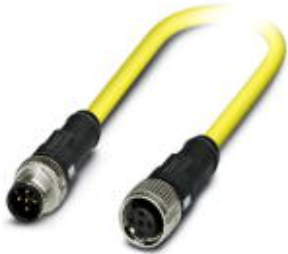
Sensor/Actuator cable, 5-position, TPE, yellow RAL 1021, Plug straight M12 SPEEDCON, A-coded, on Socket straight M12 SPEEDCON, A-coded, Cable length: 0.5 m
