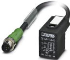
Sensor/Actuator cable, 3-position, PUR halogen-free, Black-gray RAL 7021, Plug straight M12, A-coded, on BI valve plug (11 mm), with 1 LED, connected with Z diode, Cable length: 0.6 m
