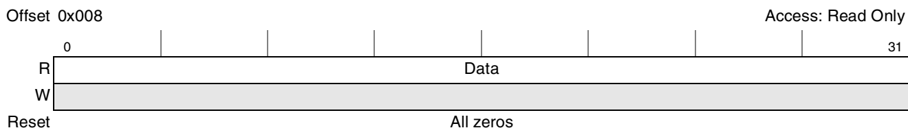
Figure 16-5. PCI/X INT_ACK Register
