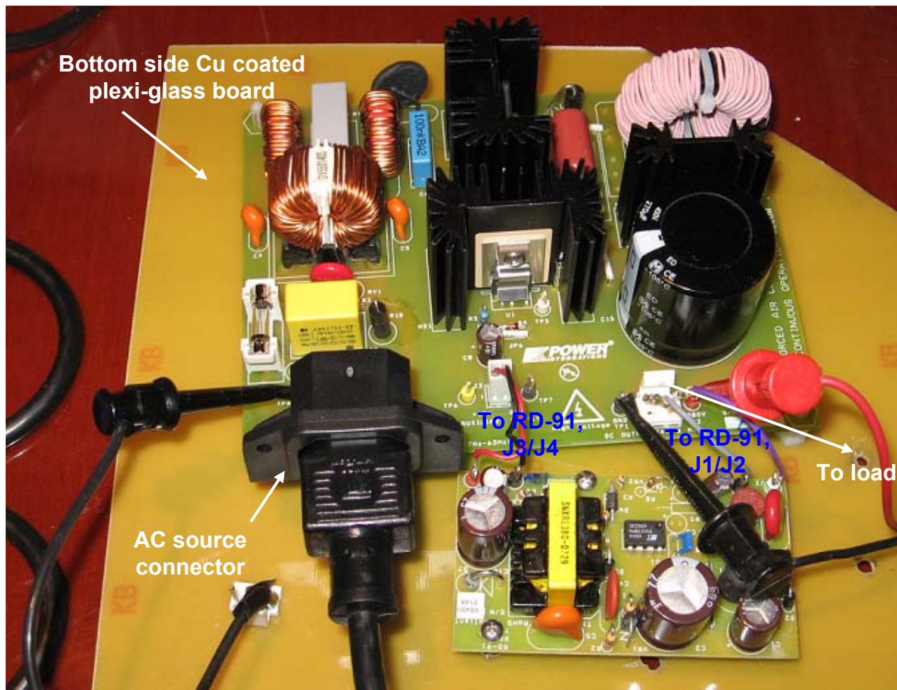
Figure 66 – EMI Test Set-up.
