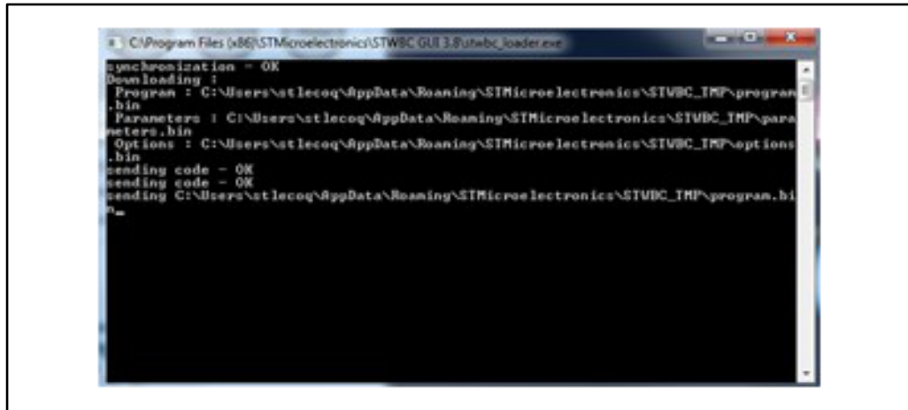
Figure 11: Firmware download progress window
