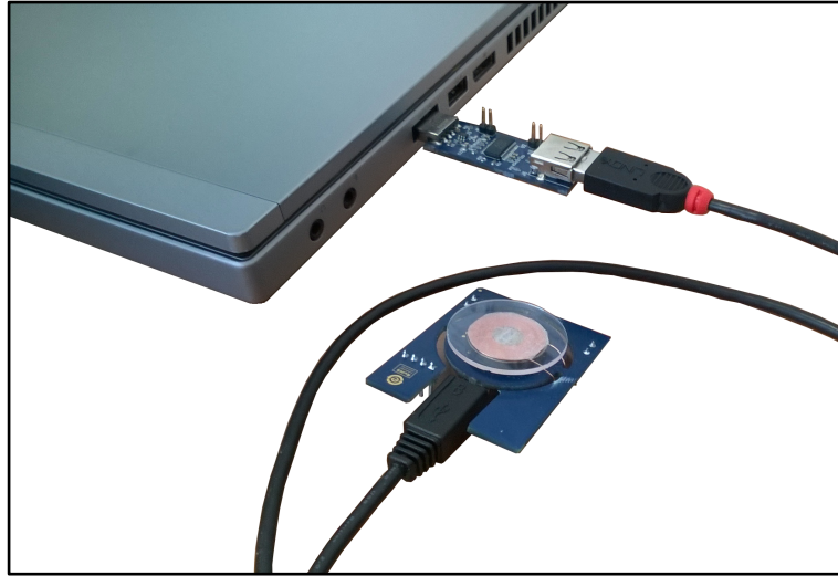
Figure 10: USB-to-UART dongle to STEVAL-ISB038V1T transmitter board connection
