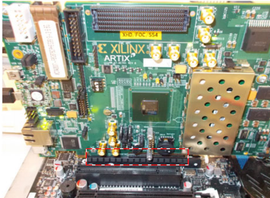
Figure 16: AC701 Board Installed in a PCIe x16 Connector
