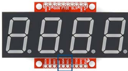
I 2 C communication requires 4 pins: SDA, SCL, PWR, and GND.
