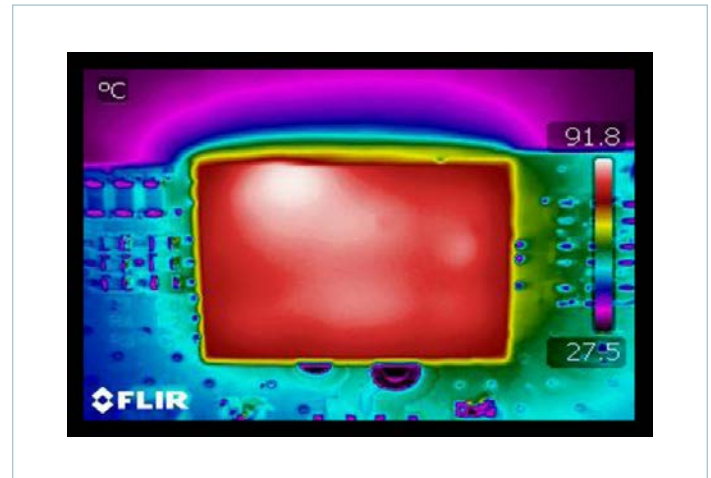
Figure 20 — Thermal Image ( V_{IN} = 28V , I_{OUT} = 10A , CR, OLFM Evaluation PCB)
