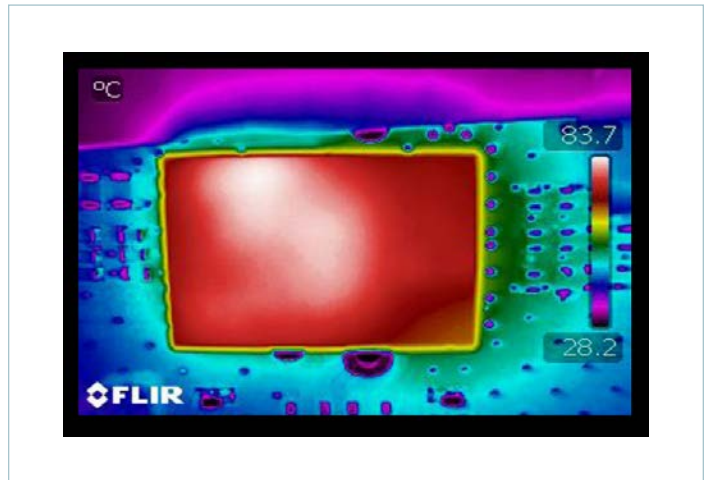
Figure 30 — Thermal Image ( V_{IN} = 28V , I_{OUT} = 4.2A , CR, OLFM Evaluation PCB)
