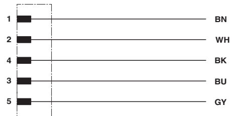
Contact assignment of the M12 socket
