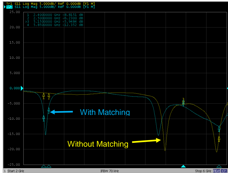
FIGURE 5.9 RETURN LOSS OF ANTENNA WITHOUT AND WITH MATCHING ON REFERENCE PCB GROUND SIZE AT REFERENCE LOCATION
