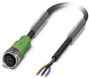
Sensor/Actuator cable, 3-position, PUR, black-gray RAL 7021, free cable end, on Socket straight M12, A-coded, Cable length: 12 m
