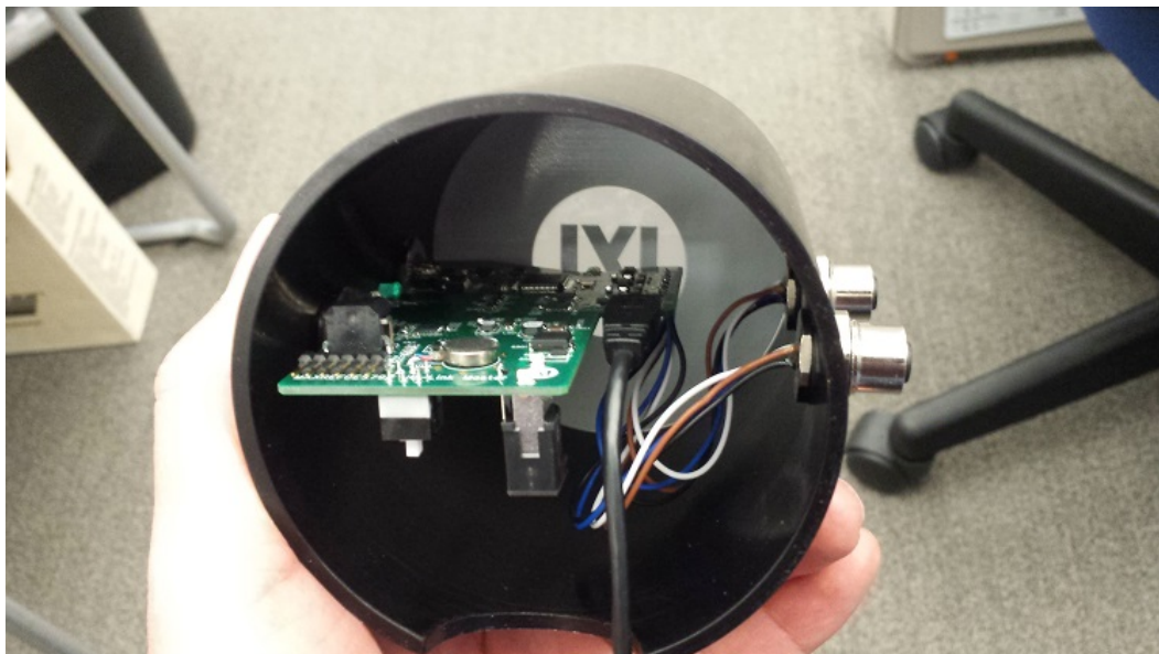
Figure 5. Connect the Micro-USB cable from underneath the MAXREFDES79# and then connect it to the PC.
