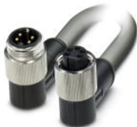
Bus system cable, DeviceNet, 5-position, PVC, Gray RAL 7001, Plug angled 7/8"-16UNF, on Socket angled 7/8"-16UNF, Cable length: 0.5 m
