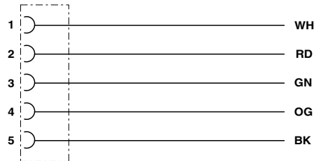
Contact assignment of 7/8" plugs/sockets, cable type 410
